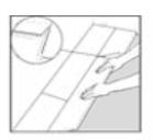
Place the second plank with the tongue side at an angle against the groove side of the plank in the previous row and the short side tite to the previous plank. Ensure that the plank is positioned on the integral locking strip of the plank in the previous row and no joint is noticed between the short sides and press forward and lay it flat at the same time slightly tap with a rubber hammer.
