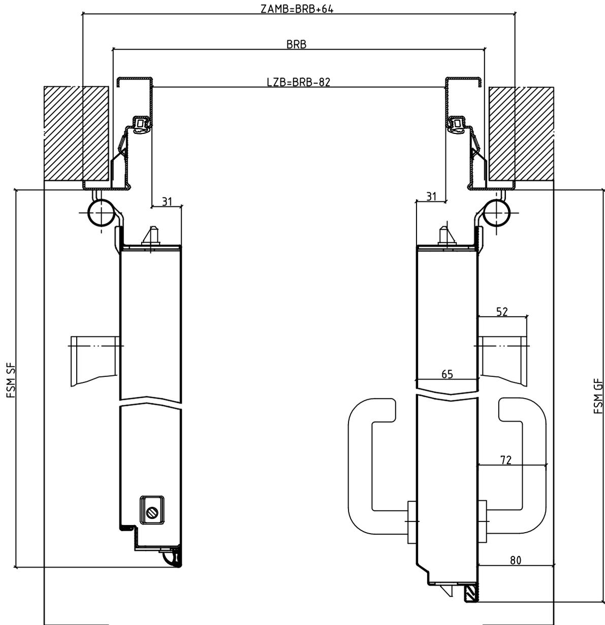
$FSM\ GF = BRB\ GF + ca.55mm$  $FSM\ SF = BRB\ SF + ca.55mm$
